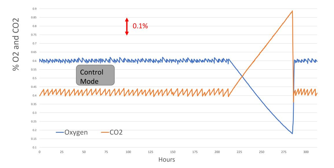
To measure the respiration and determine the RQ the control mode is halted and the increase of CO2 and the reduction in Oxygen is tracked and recorded.
