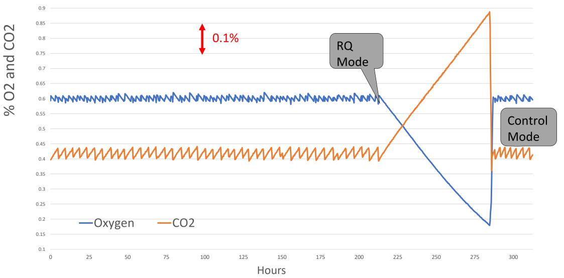
This RQ mode is left to run for a pre-set period of time equivalent to a change of approximately 0.1% Oxygen.
